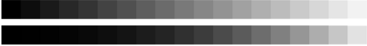
Figure 5.1: A equally-spaced gradient in sRGB space (top) and an equally-spaced gradient in linRGB, converted to sRGB for display (bottom)
